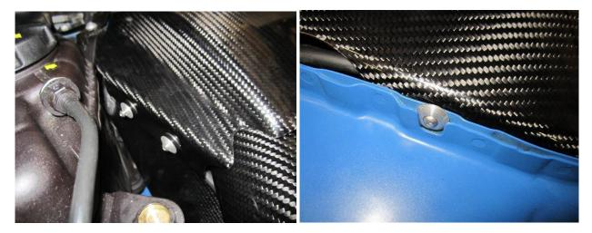
20. Re-attach the air breather to the longer carbon fibre intake pipe.
