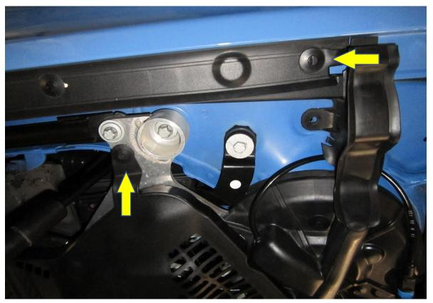
4. On both sides of the vehicle, use a 10mm socket to turn the fasteners 180 degrees to remove the plastic covers.
