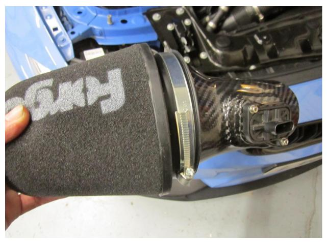
**18**. Fit the inlet pipes into position and tighten the hose clamps; again ensuring not to over tighten as this could damage or crack the carbon fibre.
