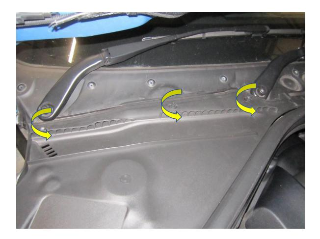
5. Using a 13mm socket, remove the 8 fasteners that hold the strut brace in position.
