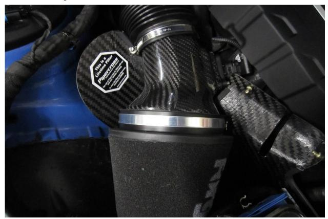
19. Place the carbon fibre airbox lids into position then tighten taking care not to over tighten as this can damage the airbox lids.
